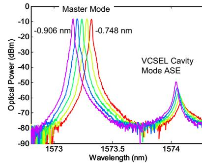
Fig. 2 (b) Optical spectra of an OIL VCSEL at various detuning values. The master laser wavelength is tuned.
