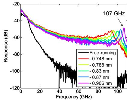
Fig. 2 (a) Frequency response of an OIL VCSEL at various detuning values. A record resonance frequency of 107 GHz is shown.
