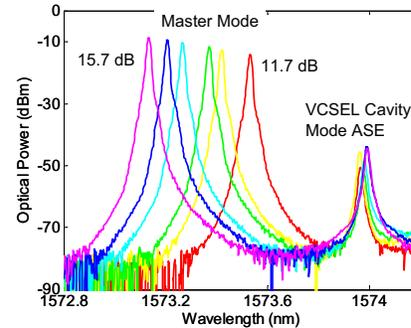
Fig. 3 (b) Optical spectra of an OIL VCSEL under various injection ratio levels. Both the power and the wavelength of the master laser are tuned.
