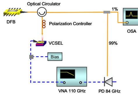
Fig. 1 Experimental Setup (VNA: vector network analyzer, PD: photo-detector, OSA: optical spectrum analyzer)
