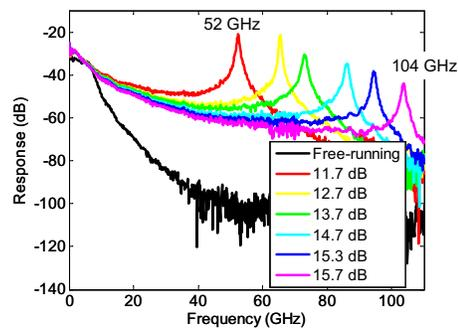
Fig. 3 (a) Frequency response of an OIL VCSEL under various injection ratio levels. The detuning is adjusted to result in a resonance peak with  $\sim 20$  dB gain for all the cases.
